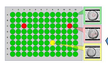
Cells gently dispensed to pre-filled 96- or 384-well microplates, and detected cell number annotated on interactive well map in Cyto-Mine® Studio software.
