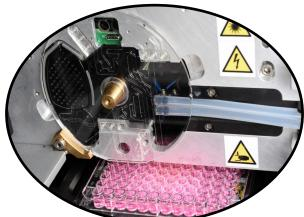
Cyto-Cartridge® and microplate loading bay
