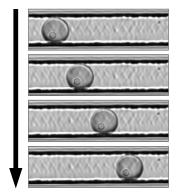
Visual verification by ultra-high speed, multi-frame optical imaging immediately prior to dispense confirms the presence of a single cell per picodroplet
